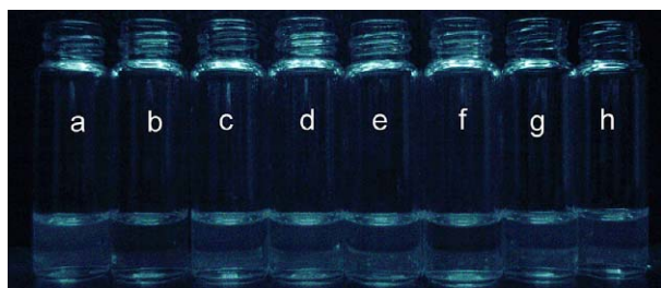
Figure 6. Visual changes for 1 upon addition of (a) no anion, (b) \text{F}^- , (c) \text{Cl}^- , (d) \text{Br}^- , (e) \text{I}^- , (f) \text{CH}_3\text{COO}^- , (g) \text{HSO}_4^- , and (h) \text{H}_2\text{PO}_4^- . Irradiation at \lambda_{\text{ex}} = 335 \text{ nm} using UV lamp.
